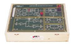
The trainer provides all necessary inputs and connection for students to study signal Sampling and Reconstruction Techniques.
