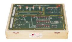
The trainer provides all necessary inputs and connection for students to study Pulse Code Modulation Transmission techniques. A communication link can be established by using PCM receiver Model ST2104.
