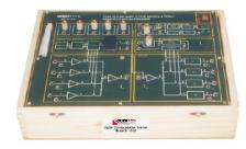
The trainer provides all necessary inputs and connections for students to study Pulse Amplitude Modulation/Demodulation techniques, Time Division Multiplexing & Demultiplexing of Signals and Signal Reconstruction.
