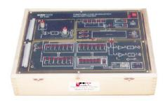
The trainer provides all necessary inputs and connection for students to study decoding and demultiplexing of data transmitted by PCM transmitter. On-Board PLL provides regeneration of Clock. Synchronization between transmitter and receiver is provided by Pseudo random code.
