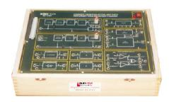
In digital communication specially operating at low frequencies or speech communications a saving in Bandwidth can be resulted using Delta Modulation and its associated techniques because this requires single encoding of sample. This Trainer covers Delta, Adaptive Delta and Delta sigma Modulation and Demodulation
