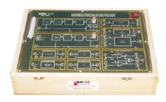
In digital communication Data Formatting is very important. The available data stream from PCM transmitter is converted into different formats best suited to individual transmission system. Various formats are covered in this trainer. Also to transmit the digital information Carrier Modulation is necessary. Various modulation techniques are also covered in this trainer.
