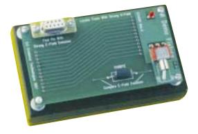
EMC Demo Fixture model CTA201 features a multitude of typical EMC problems: a high frequency clock with sharp edges, questionable grounding, poorly laid out and unterminated traces with distributed inductance and capacitance, poor ground returns, etc.
